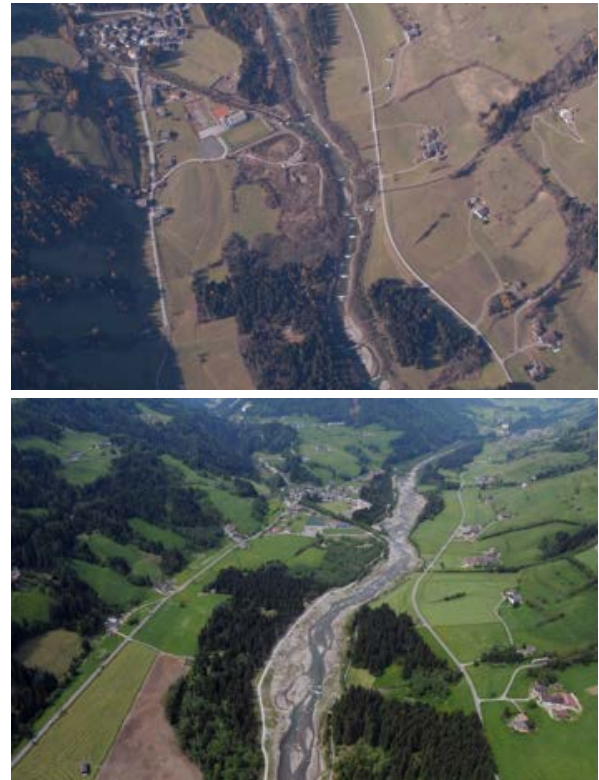
Figure 16: River widening – Mareiterbach; before-after, South Tyrol (©Autonomous Province of Bolzano/Bozen, Civil Protection Agency)
