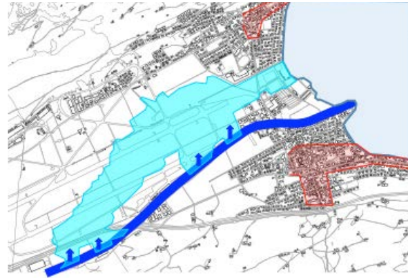
Figure 40: Situation after constructional adaptation with four floodable dyke sections, reduced residual risk area and back dykes for the protection of the settlements (©Tiefbauamt Nidwalden, 2006)
