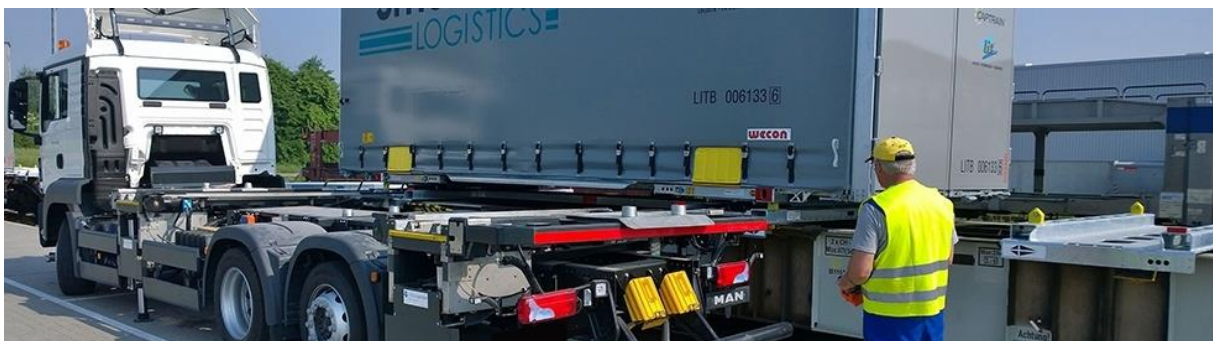
Rail/road transshipment according to InnovaTrain AG, source: www.innovatrain.ch
