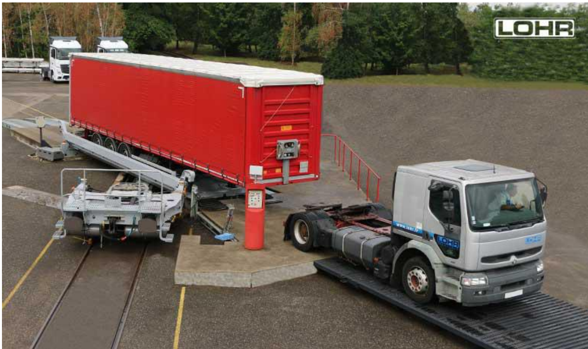
Modalohr wagons on the Alpine rolling motorway, source: Innovation in rail freight transport in France ( L'innovation dans le transport ferroviaire de fret en France ), CGEDD (French General Council for the Environment and Sustainable Development), September 2016
