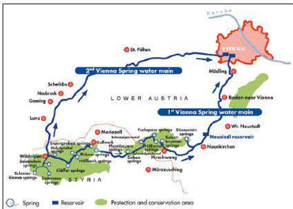
Fig. 17 - Drinking water production areas in the city of Vienna
