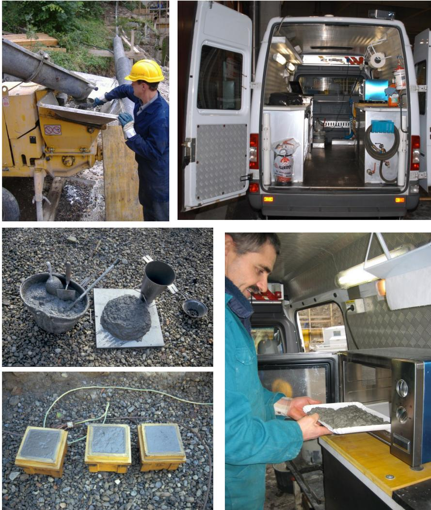
Mobile unit for quality control of building materials during the early contraction phases - a contribution to a prolonged durability and an increased reliability of protection structures (Autonomous Province of Bolzano)
