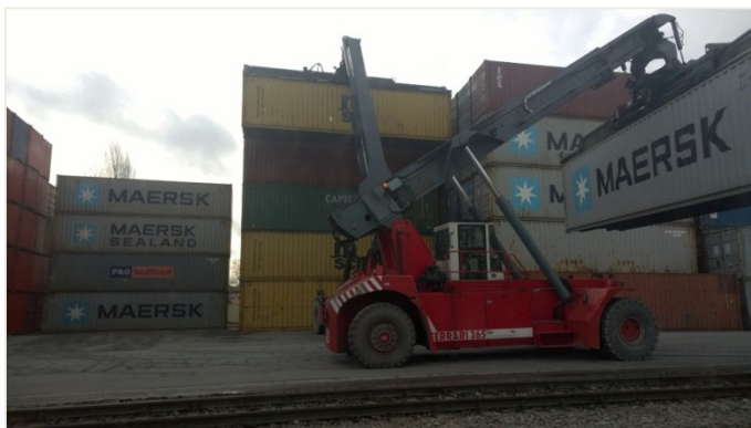
Figure 24: Transshipment of container with reach stacker 106
