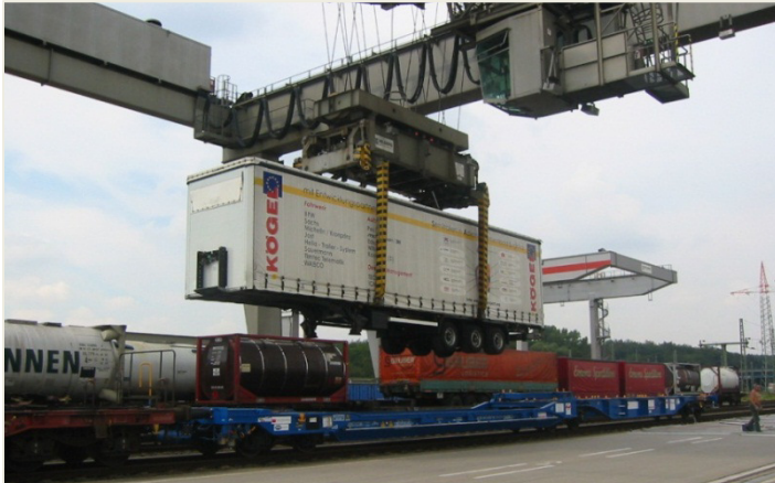
Figure 23: Transshipment of a craneable semitrailer with help of a gantry crane 104
