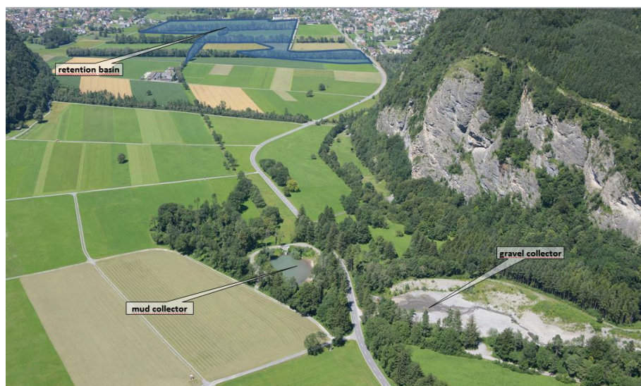
Fig. 23: Overview of Sediment traps at Andrùfe and retention basin at Balzers
