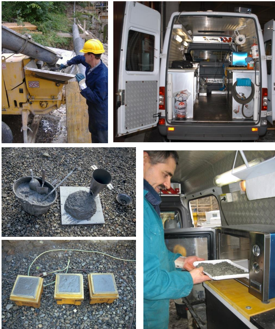
Mobile unit for quality control of building materials during the early contraction phases - a contribution to a prolonged durability and an increased reliability of protection structures (Autonomous Province of Bolzano)
