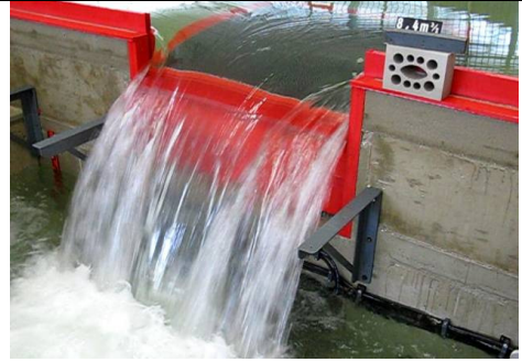
Figure 3: Position of shaft power plant within the weir © Department of Hydraulic and Water Resources Engineering TU München
