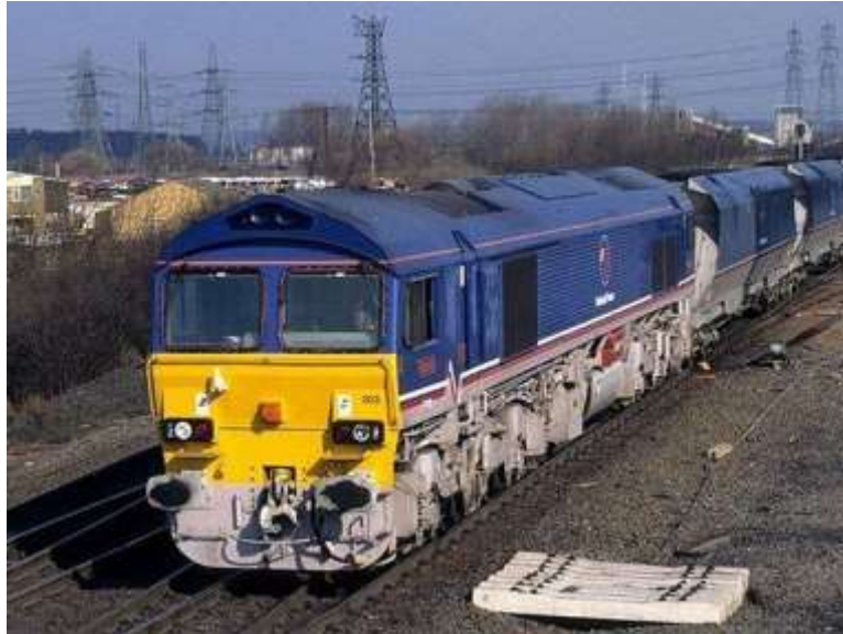
Photo 16: Janney Automatic Coupling in Great Britain in a swiveling version which can be compatible with the screw coupler. (Source: Ivan Beltramba)
