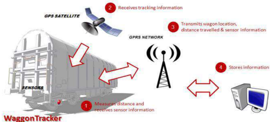
Figure 2: Example of digital equipment of freight wagon
