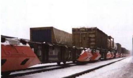
Photo 3: Bogie skirts for noise protection
