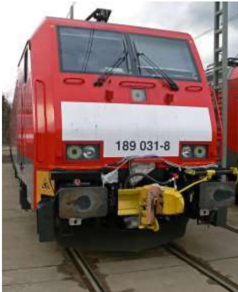
Photo 9 Locomotive with C-AKv coupler Photo 10: Coupling with conventional screw-coupler
