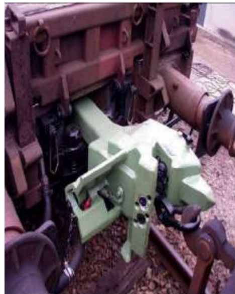
Photo 9 Locomotive with C-AKv coupler Photo 10: Coupling with conventional screw-coupler
