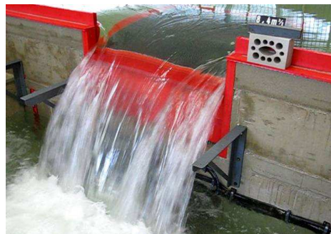
Figure 16 and Figure 17: Position of shaft power plant within the weir © Department of Hydraulic and Water Resources Engineering TU München
