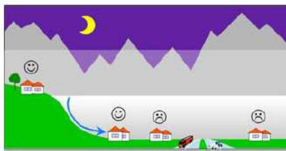
Fig. 11b During clear nights the exhausts are caught in the inversion near the valley bottom. Places close to the foot of the side slopes benefit from down-slope winds (blue). Plateaus often rise above the polluted inversion layer and remain in the residual layer of the previous day.
