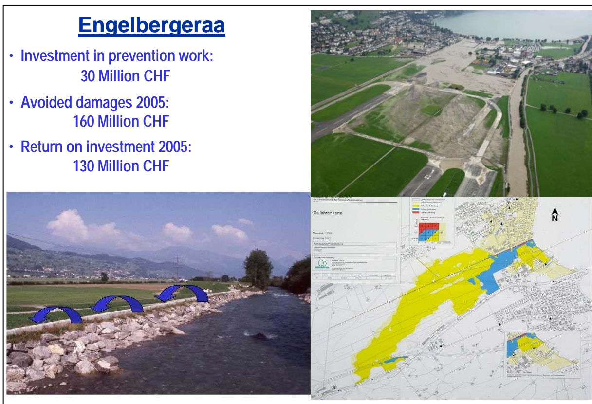
Figure 11: Surveys of defence measures must always consider what happens in the case of overload. In this example, in a flood situation the water flow through the urban area is controlled to minimise damage. Studies have shown that the measures in place here averted considerable damage during the 2005 floods (photo: Swiss Air Force, Switzerland).
